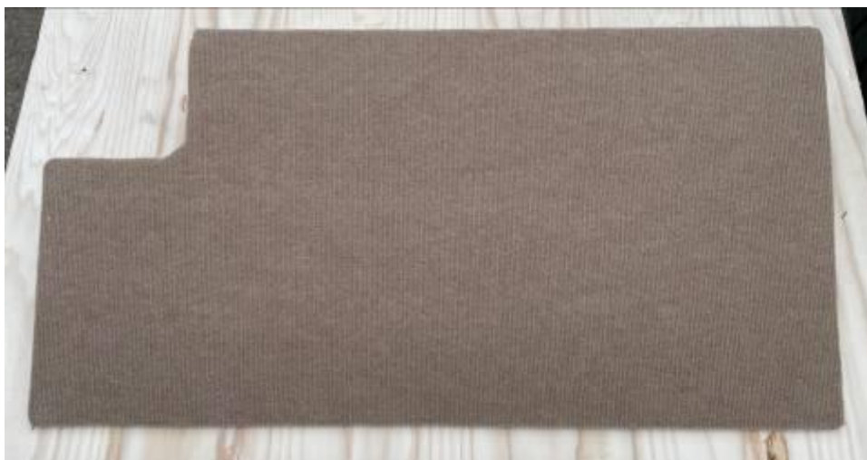
Rear board with corner cut-out for fuel filler pipe.
