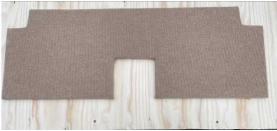
Front board cut out for seat belt brackets and body support brace.
